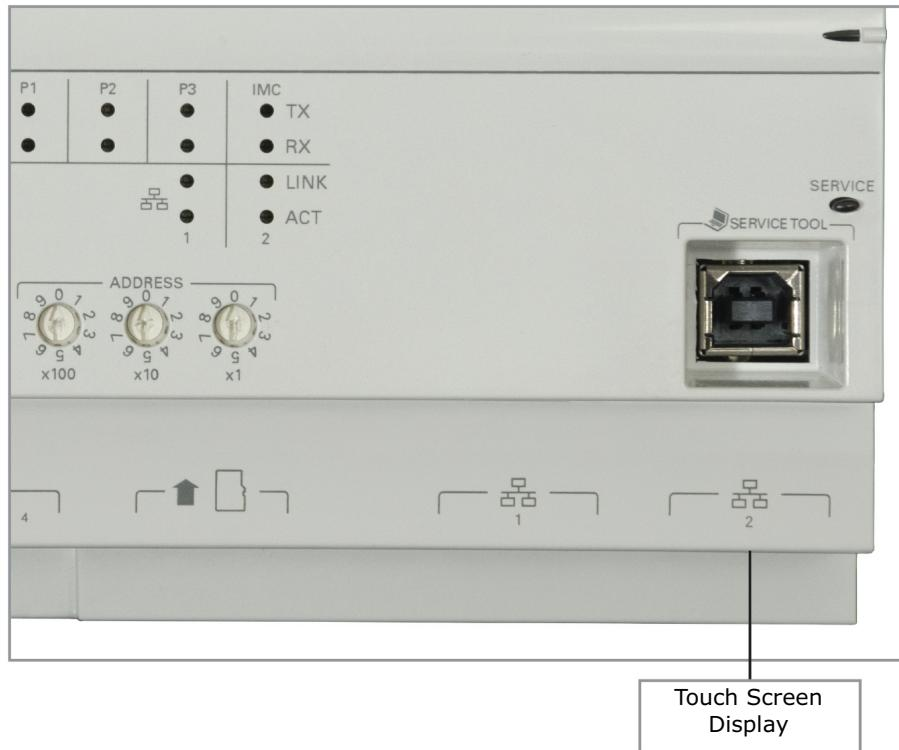
**Note:** Ethernet Port 2 is for use with the Touch Screen display only. Communication to other devices is not supported.
