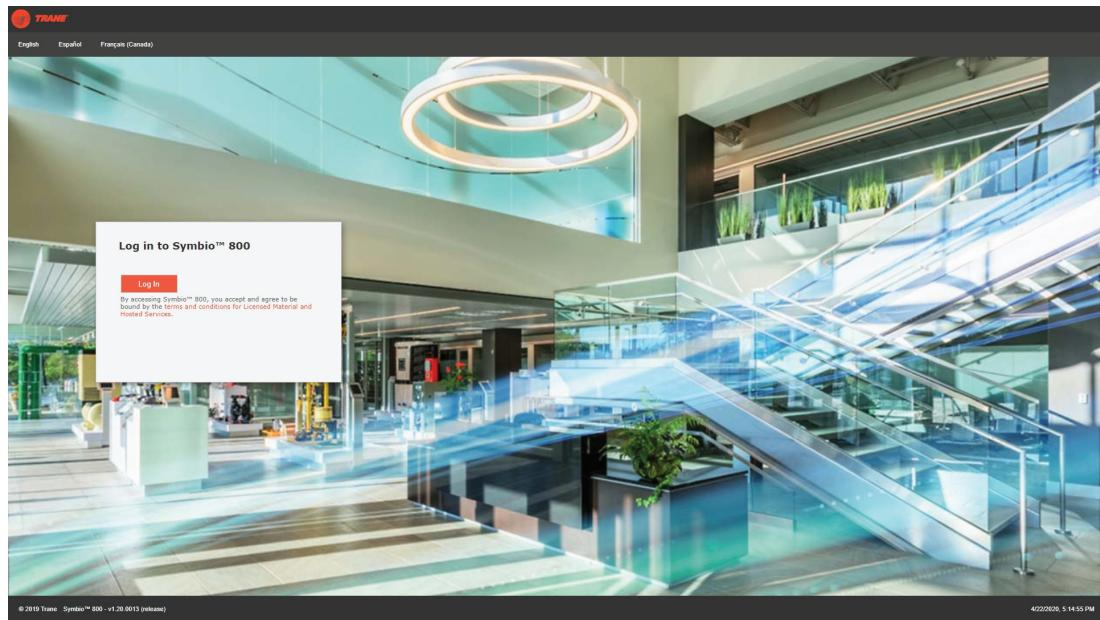
**Note:** The Symbio™ 800 web interface can only be viewed using the USB connection. Ethernet port 1 and Ethernet port 2 will not allow access to the Symbio™ web server to meet IT security requirements.
