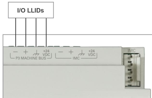
Figure 17. IMC link terminations for optional Air-Fi and expansion module (XM30)
