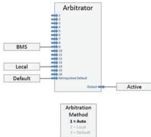
When the Arbitration Method is selected as local, the BMS value is ignored and local value is used instead. Though the arbitration logic still considers all inputs, any values sent by the BMS are effectively ignored.
