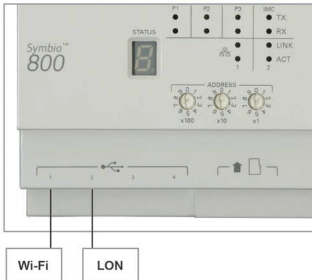
The controller automatically detects devices on any of the ports (not port specific). The controller ships with all ports enabled, but they can be disabled via the Web interface.
