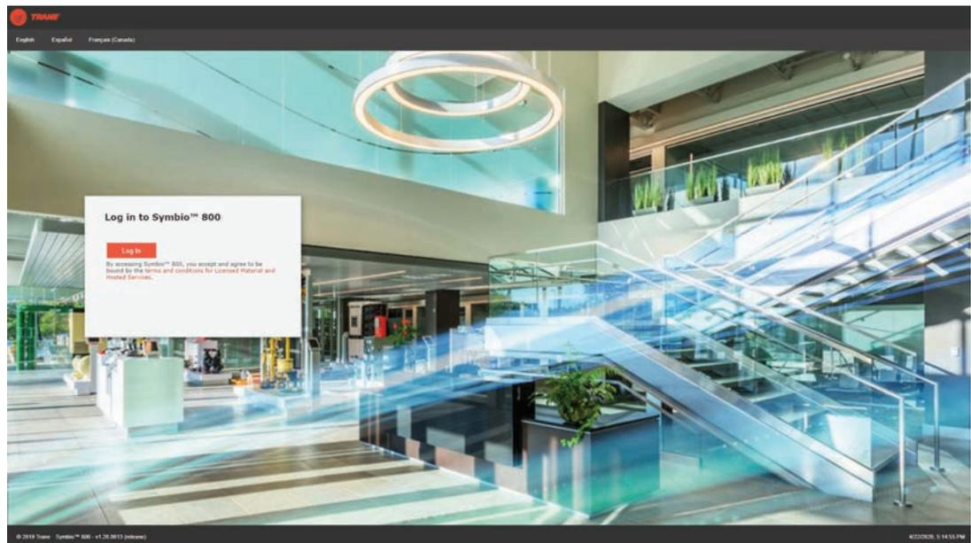
**Note:** The Symbio™ 800 web interface can only be viewed using the USB connection. Ethernet port 1 and Ethernet port 2 will not allow access to the Symbio™ web server to meet IT security requirements.
