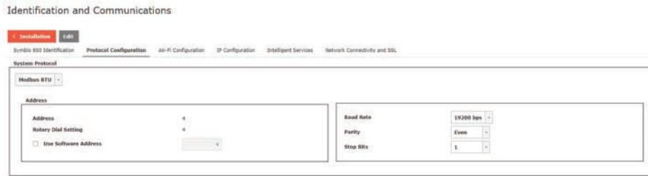
1. Set the Communication Protocol drop down to **Modbus RTU**.
